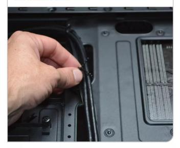
STEP 5 Keep airflow in mind and don't cover any case fans or coolers with a cable if at all possible. The Component placement within a system is also important. Drives, graphics cards and other expansion cards should be positioned in such a way that their cables, or the components themselves, don't interfere with one another. Don't be afraid to move a component if needed.
