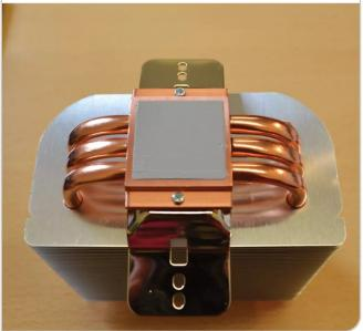
Before fitting the actual Freezer 7 cooler, we needed to remove the fan from it. Your cooler may not require this but many do as it helps give access to the screw fitting that secures the cooler to the mounting plate. The Freezer 7 fan simply clips on, so removing it is easy. If you remove the fan from your cooler before fitting it into place, make sure nothing will impede it.
