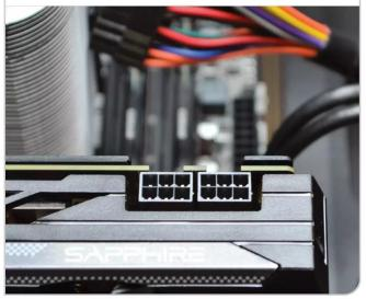
Press the card down from the top, evenly but firmly, until it clicks into place. Slide or flip the socket catch to secure it. Check that all of the ports such as HDMI, DVI, etc. are accessible from where they protrude from the expansion slot at the back of the case and then use the screws you removed to take out the blanking plates to secure the card to the edge of the slot.
