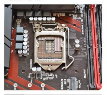
The arrow shows you which way the chip sits in the socket (arrow to arrow). Intel processors also have a small indentation on each edge, which further helps you to line it up in the socket. Holding the CPU carefully by the edges, lower it it into place in the socket. Ensure it is seated correctly, with the arrows and the notches lined up and in place.
