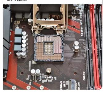
You can now remove the plastic cover on the CPU lock, lower it down over the seated CPU and slide it into position. The exact locking process may vary slightly, even between the Intel family of CPU's, but most will slide the locking frame under a metal plate or raised washer. Firmly press the locking bar into the locked position. Your processor is now safely installed onto the board.
