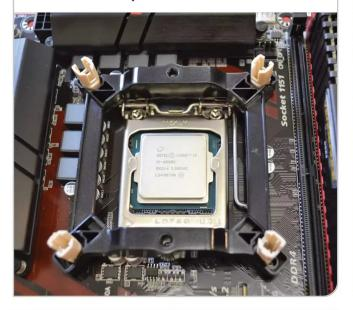
There should always be a layer of thermal paste between the bottom of the CPU cooler heatsink and the CPU. Thermal paste helps to improve heat dissipation by filling the tiny gap between the heatsink and CPU. Our cooler has a layer of thermal paste pre-applied but not all do. You can buy thermal paste applicators cheaply online or at PC stores.
