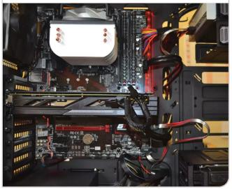
Some cables, such as the front panel audio, branch into two connections when you only need to use one. This usually means that a second connection branches off just before the main cable terminates. Fold the excess cable back on itself and tie it down to the main cable so it's out of the way. Do this for any other cables around the case, such as the PSU's SATA power cables.
