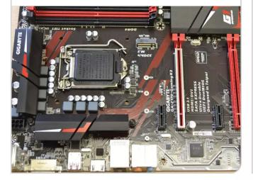
The process for fitting an AMD or Intel CPU is similar, but there are some physical differences between the two processor types, not least the arrangement of the contact pins. We are using an Intel Core i5 6600k CPU for our build and we will concentrate on that process. See further down the guide to see specific AMD CPU installation advice and precautions.
