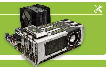
Make sure there is no cover on the card connector and then carefully lower it into the PCIe socket.
