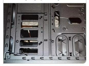
Once the cable bundle is fed through the fixed side panel, we can start feeding the individual cables into wherever they are needed. They can then be fed back through any convenient hole, so that the connectors are back in the main compartment and ready to be plugged in. When you are doing this, take a moment to ensure that the removable side panel will fit back on with the cables here.
