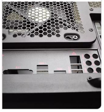
Lay the case down flat if it isn't already and lift the motherboard carefully in. Whenever you are going to touch the motherboard, especially the exposed connections on the back, make sure you are wearing an anti-static wristband and clip or that you discharge any built up static electricity in your body by touching a large metal object, like a desk.
