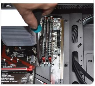
During the preparation of the case, you should have positioned the metal risers in the correct holes based on the form factor of your case and motherboard. Check to see if the holes on the motherboard now line up with your risers and reposition if needed. Identify the motherboard fixing screws that are supplied.
