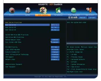
Use the arrow keys to select the BOOT tab. System devices appear in order of priority. BIOS settings allow you to run a boot sequence from a floppy drive, a hard drive, a CD-ROM drive or an external device. You may configure the order that your computer searches these physical devices for the boot sequence. The first device in the order list has the first boot priority.
