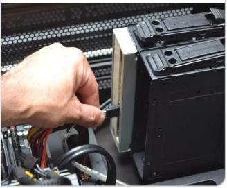
You can now replace the front panel of the case and adjust the position of the optical drive, if needs be, by loosening the fixing screws slightly and using the slots to slide it back or forward. If you have a second optical drive to fit and if your case features a second bay, repeat steps 1-4. There are several other components that can be fitted into a 5 1/4 in drive bay, such as fan controllers.
