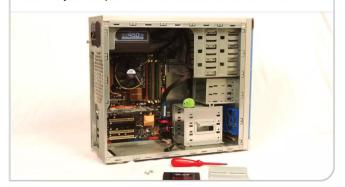
Note that one end of the SSD has the connectors on it. You'll need to position the device so that your power and SATA data cables can reach these connectors.
